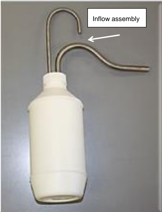
Figure 17: Stage sampler bottle with inflow assembly
