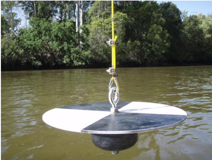
Figure 8: Secchi disc attached to 3kg weight and tether
