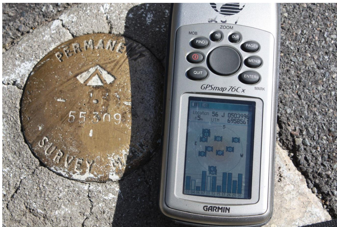
Figure 6: GPS next to permanent survey mark 55309
