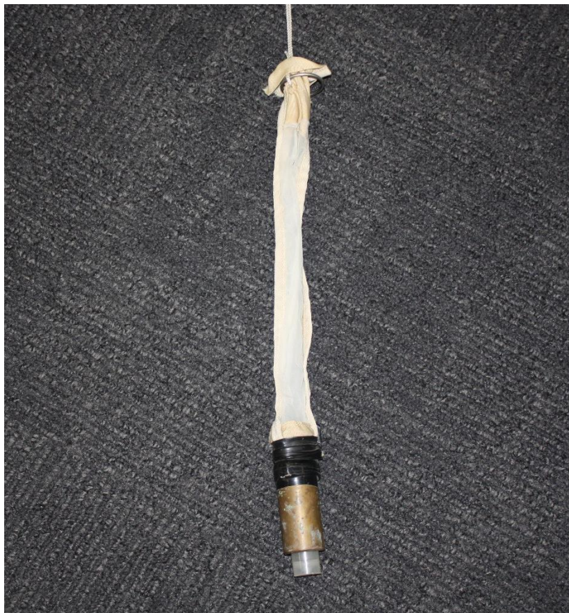
Figure 45: Example of a net used to sample stygofauna, with collection vial attached to bottom of net
