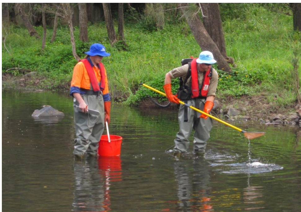
Figure 50: Backpack electrofishing being undertaken, with assistant carrying bucket and ready to take notes on catch
